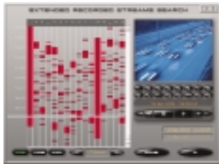
The Image Find feature of the DVN 3000 allows you to select a specific camera, date and time to pinpoint an exact image.
